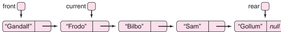
FIGURE 16.19 A linked list: front references the first node, rear the last, and current holds the address of an arbitrary node
