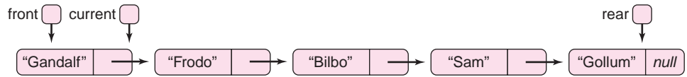
FIGURE 16.20 A call to reset() sets current equal to front and hasNext() returns true
